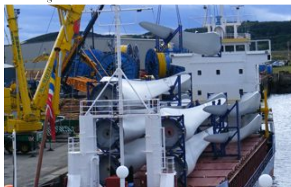
Unloading turbine blades
